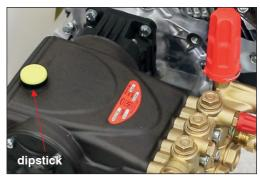
**OIL LEVELS -** Check oil levels on the sight glass of the pump, the oil should be half way up the sight glass - ensure machine is on a level surface.
