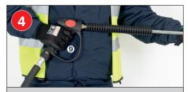
• Pull the trigger on the gun and lance assembly, the Wheelbarrow tank pressure washer is now ready to use.
