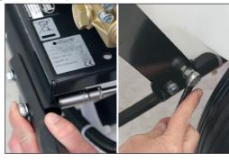
**⊙** HOSE REEL & HOSE - Assemble the hose reel and high pressure hose following instructions inside the box then attach this to the hose reel bracket with supplied bolts.
