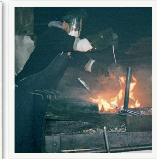
Below: Steel as it travels through the various stages of production to become a trowel Bottom Left: Initial cutting of the forged steel bars Bottom Center: Forming the shank Bottom Right: Part of the heat treatment process
