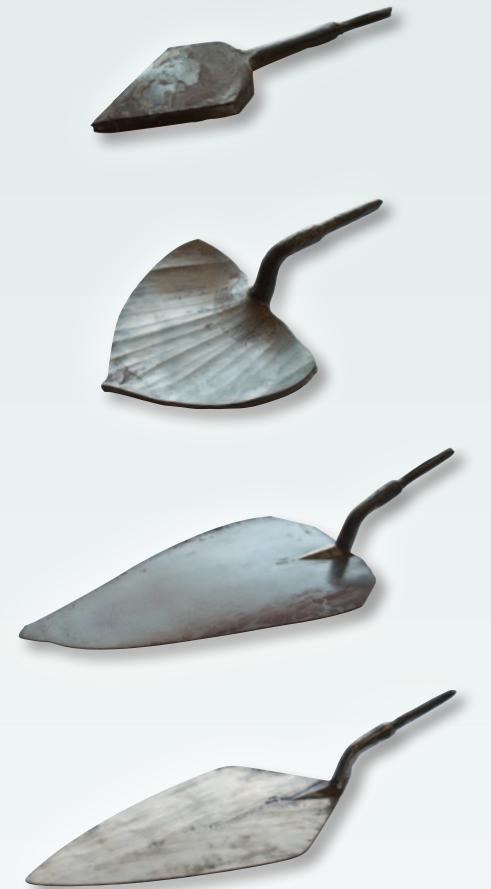
Below: Steel as it travels through the various stages of production to become a trowel Bottom Left: Initial cutting of the forged steel bars Bottom Center: Forming the shank Bottom Right: Part of the heat treatment process
