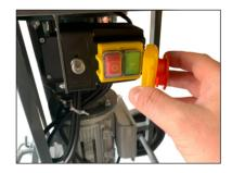
To restart the mixer, you need to do the above again before restart it by pushing the green ON button at the main switch. This switch is below the emergency stop button casing.
