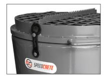
Before you start the mixer, the Grid Lid has to sit on the mixer drum and be secured by the Rubber Strap. When you unlock the Grid Lid and lift it little bit, the motor will be shut down.
