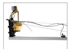
Adjustable tensioning device avoids beam deflection.
