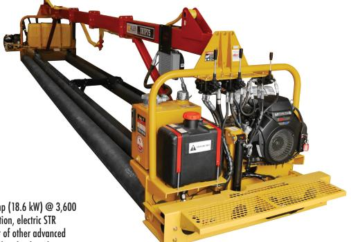
Powered by the Honda iGX800 with 24.9 hp (18.6 kW) @ 3,600 rpm (SAE J1349) with electronic fuel injection, electric STR governor, drive-by-wire control, and a host of other advanced features help to maximize productivity and make the job easier.
