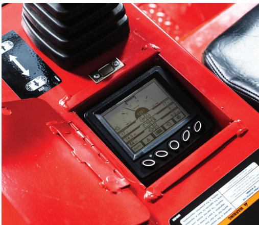
Digital read out shows accurate fuel levels, temperatures and more.
